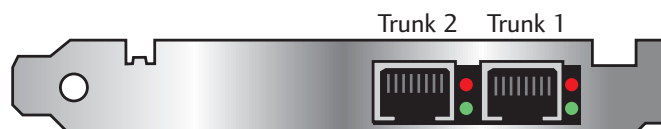
Figure 5-4: Trunk Status LED Locations
