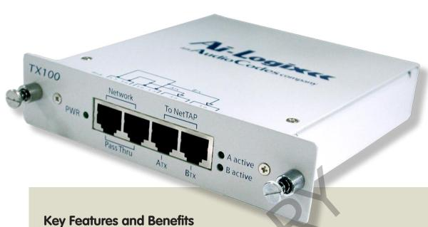
The TX100 provides two active receive connections to IP network monitoring equipment such as an AudioCodes IPX and IPR or AudioCodes IPM260. It can be placed anywhere in the configuration between two network devices. Designed with passive circuitry, the TX100's access point does not introduce and point of failure in the network even if there is no power to the device.
